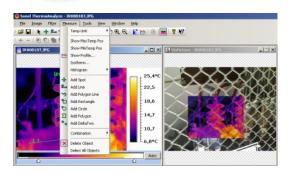
InfraFusion technology – thermograph is overlaid on a part of visual image, in a palette chosen by the user. The thermograph is overlaid with selected transparency for optimized presentation and marking of images, particularly when visual comparison of the area from the thermograph with the details on the visual image is difficult.
