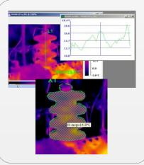
Determine and read the minimum, maximum and average temperature for the whole area or for each selected area. Select the section (straight o broken line) for which the averaged temperature can be determined and an automatic temperature distribution profile can be made.
